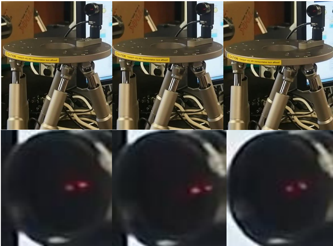
Figure 9. The laser beam is centered in the first panel, off-center in the second panel, and centered again in the third panel after the hexapod adjusts the lateral sensor's position.
